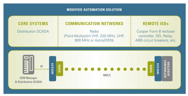
"Using the ACE3600 and the IGIN software suite, utilities can break the 80/90 site traditional bottleneck. On a single 900 MHz MAS paired channel, over 200 remote sites with significant amounts of data exhibit round trip control times of only a few seconds."
